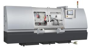
The machine is based on the standard 'T' configuration with the base being formed by a high quality Meehanite casting, designed in such a way to ensure high stiffness and damping properties are inherent in the machine.
