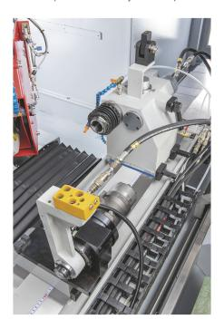
The swing down dressing system, which is freely positioned along the Z-axis table, combined with the Q-Soft operating system software significantly reduces the complexity of setup and changeovers between jobs, equally the operator training requirements are kept to a minimum.
